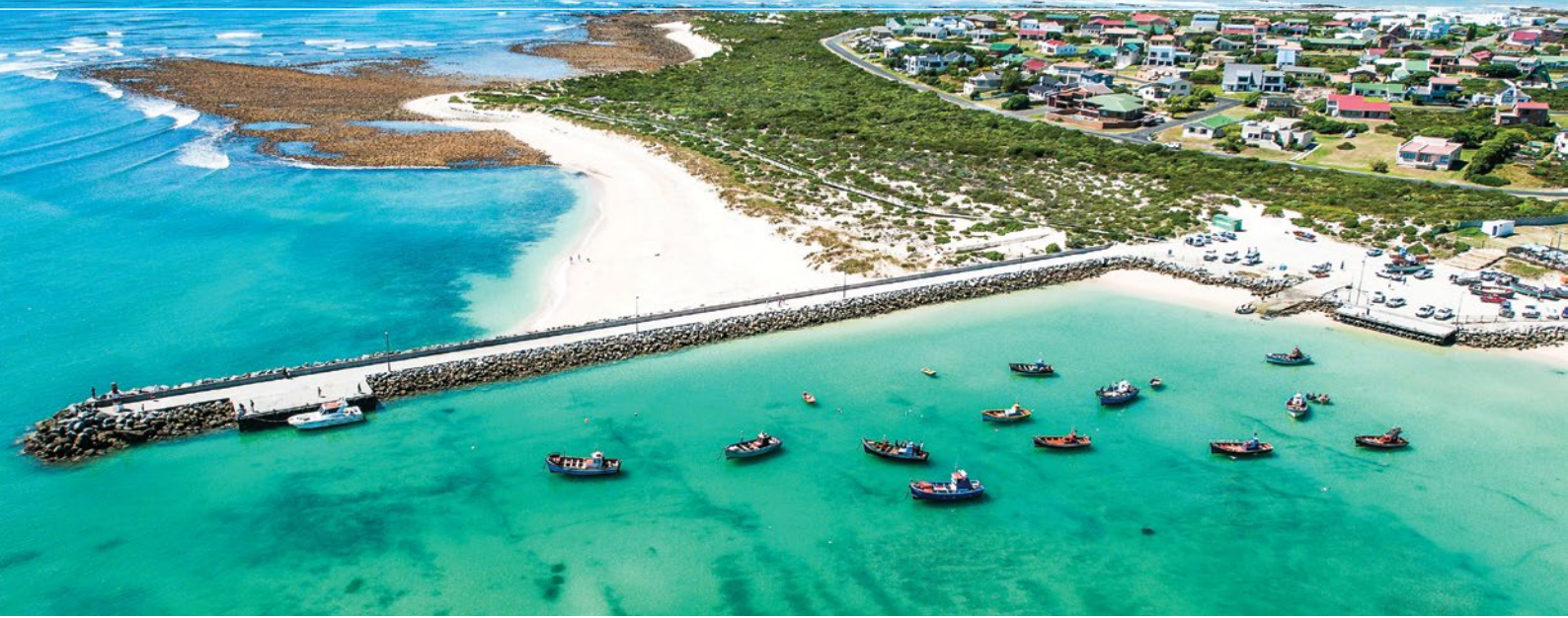
This aerial view of the Struisbaai village and harbour shows well-planned coastal development behind setback lines, but also how the building of artificial structures like the breakwater wall can affect natural sand movements. © Peter Chadwick.
