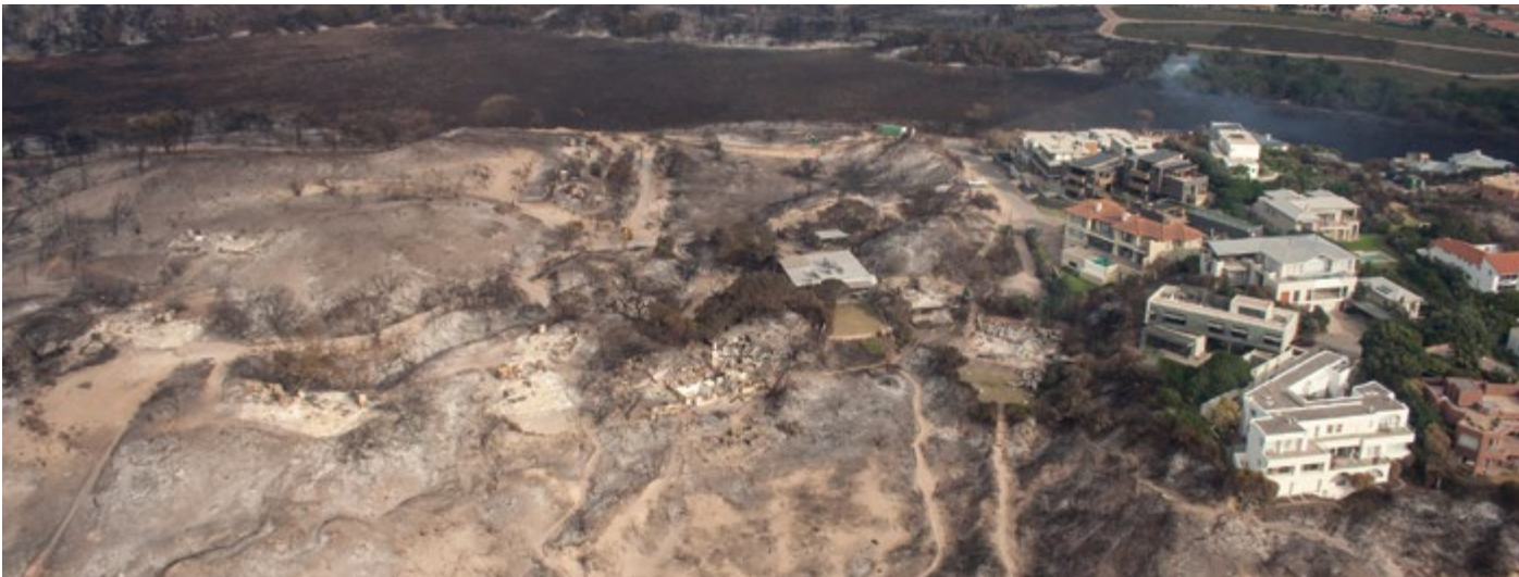
Above: Homes in White Location (an informal settlement above the town of Knysna) were lost due to direct heat and flame exposure, structure-to-structure ignition and ember attack. If you follow the path of destruction, imagine the intensity of the wildfire spreading up the slope and impacting on the homes, especially on the edge of the community.
