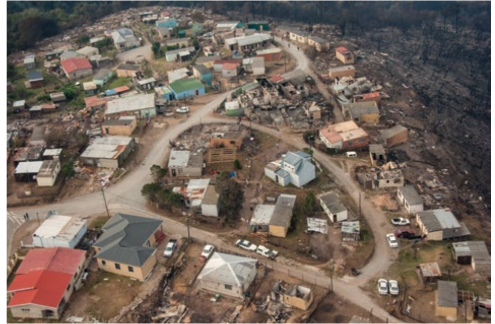
Above: Homes in White Location (an informal settlement above the town of Knysna) were lost due to direct heat and flame exposure, structure-to-structure ignition and ember attack. If you follow the path of destruction, imagine the intensity of the wildfire spreading up the slope and impacting on the homes, especially on the edge of the community.
