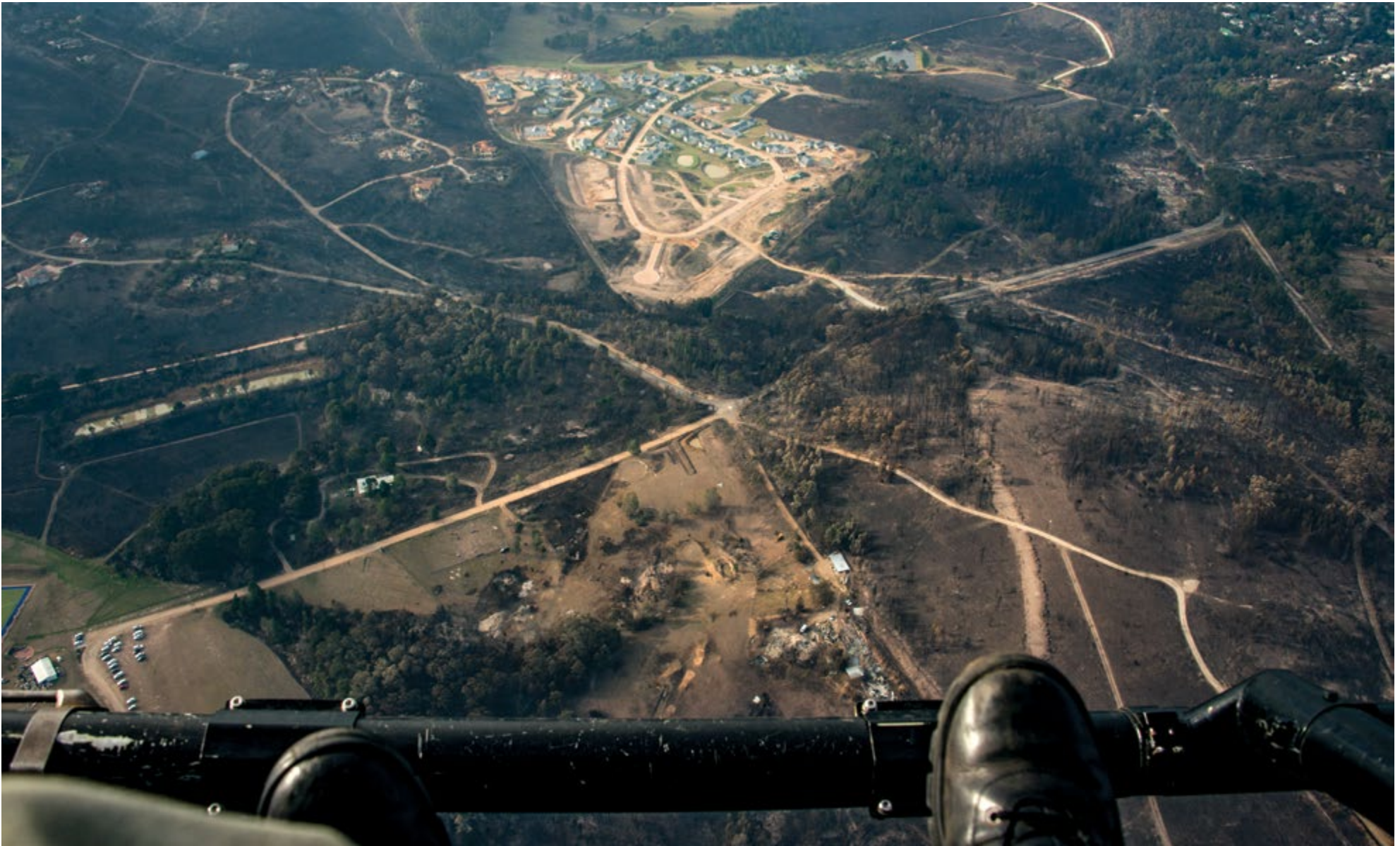
Above: The green lawns in the newly constructed complex in the centre of the image show how effective a Wildfire Resilient community could be. The fire moved around this complex as water does around a barrier, no homes were damaged or lost in this complex due to the lack of dense vegetation within it or close to the homes. The homes were also more secure against ember attack being newly constructed. This occurred purely by chance but it does highlight how important building with wildfire risk in mind is and how this could affect any future mass evacuations such as that which took place in Knysna on the 7th June 2017.
